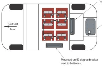
Mounted on tub above rear axle.
