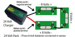
Each of the battery packs shown so far have only had batteries connected in series. Notice how the positive post (terminal) of one battery is connected to the negative post (terminal) of the next battery. The voltage of each battery adds to create a larger total battery pack voltage.
